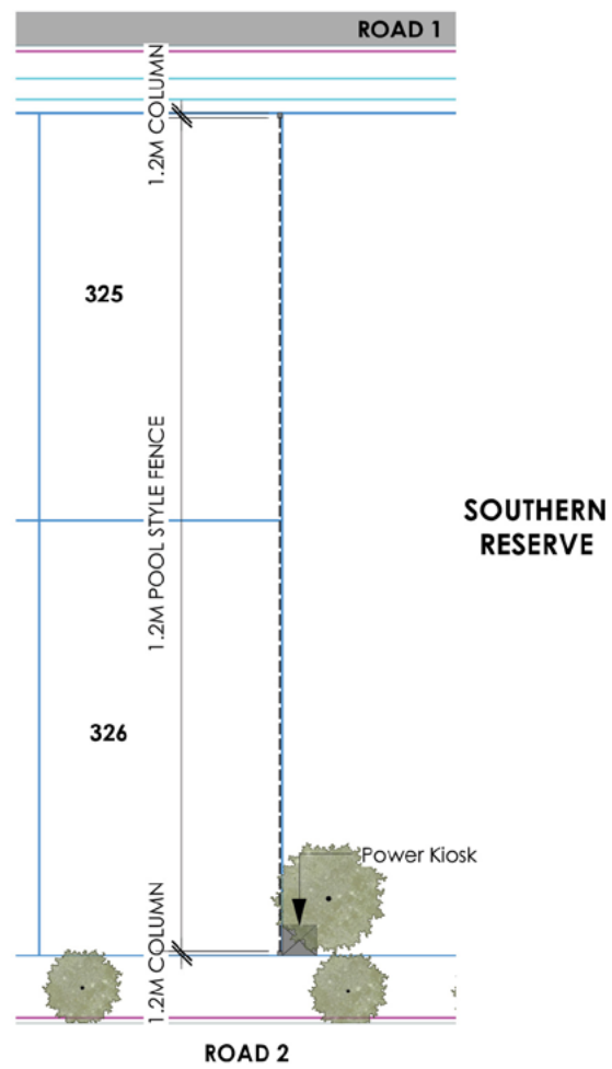
NORTHERN AND SOUTHERN RESERVE - TYPICAL BOUNDARY FENCING - ELEVATION 1:100
