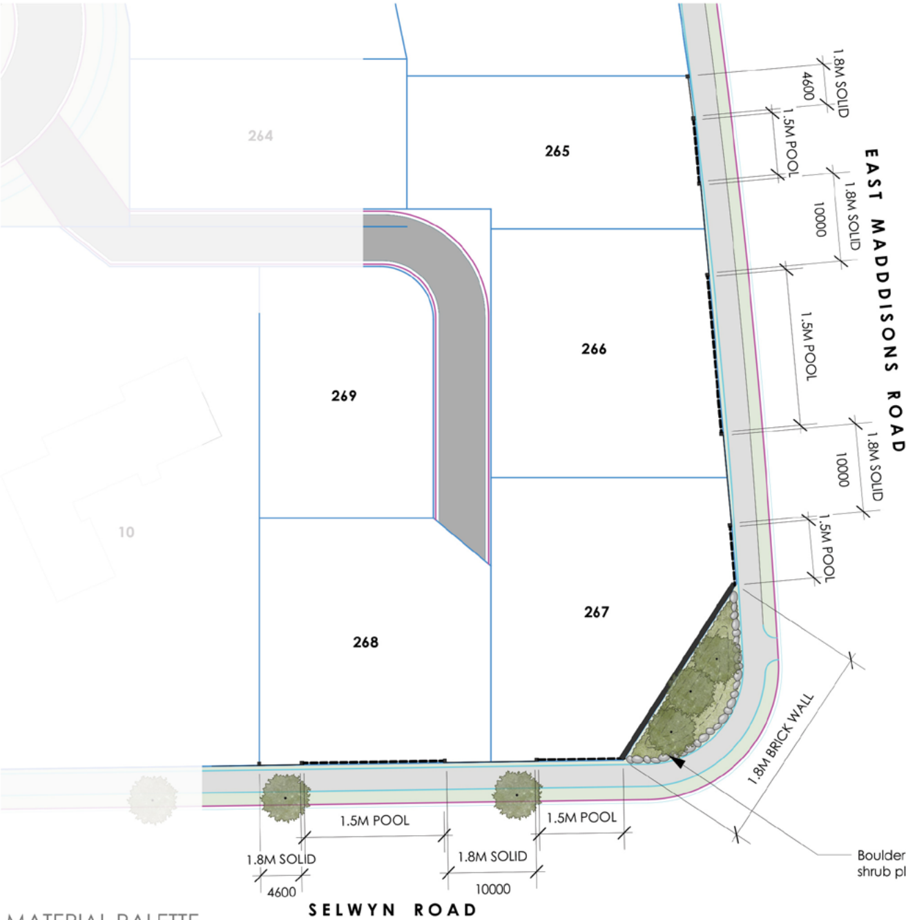
LOT BOUNDARY TREATMENTS - TYPICAL PLAN 1:300
